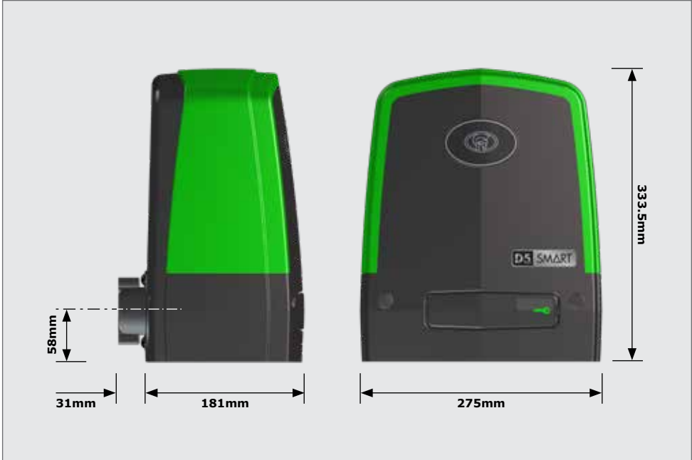
FIGURE 1. D5-EVO SMART PHYSICAL DIMENSIONS
