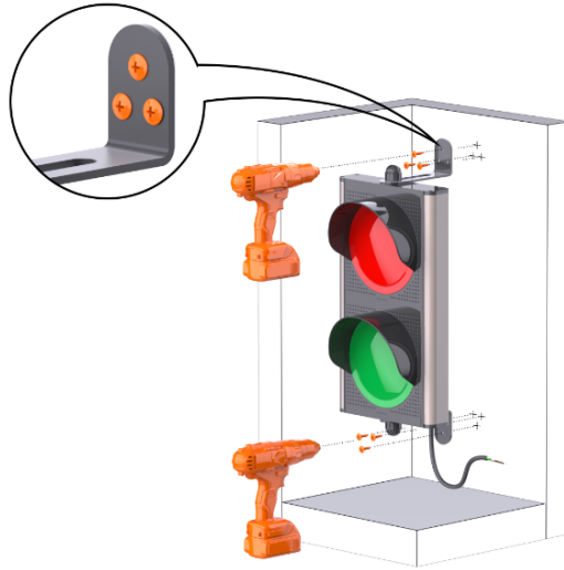
Figure 7 - TRFL Wall Mounting
