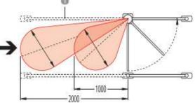
Anti-panic features: In an emergency, the gate can be pushed open to allow personnel to exit.
