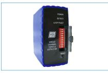
**LD100 Loop Detector** With high noise immunity, which prevents interference from outside sources, and eight sensitivity settings and ASB (automatic sensitivity boost).
