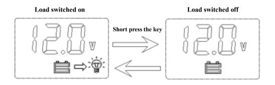
Note: As load start is a type of soft start, display of the load icon on the LCD screen will be delayed after the load is switched on.
