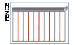
A fence is often used to stop pedestrians gaining entry under the boom pole. In areas where there are numerous pedestrians it is advisable to also fit a warning device such as a buzzer or flashing light.
