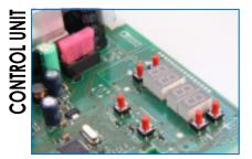
Easy to set up large LCD display with multiple functions. Speed control, ramp up and down, safety sensing are all stored in the memory. No relays on board make the unit very reliable.
