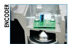
The advanced innovative and precise Absolute Encoder is assembled on the slow shaft of the motor. It monitors the safety sensing circuit hundreds of times a minute allowing for instant reverse of the boom pole.
