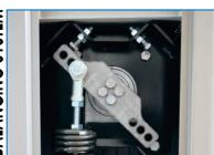
durable, high quality springs are supplied in different sizes to efficiently balance the boom pole. The springs are rated for over 3 million operations.
