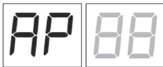
The command signal status is shown on the left hand side of the display for 5 seconds, ONLY when the respective command signal is active (AP, CH, PP, PE, OR).
