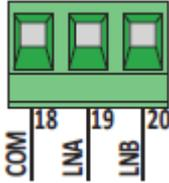
RS485 serial communication cable connection (3 x 0.5 mm- max. length 20 m) for installation of two MASTER / SLAVE opposing barriers (from firmware version n6 13 or later).
