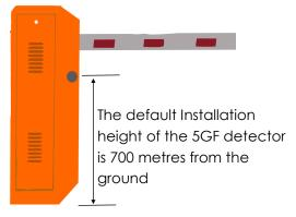
Fig.5 Detector Installation Diagram
