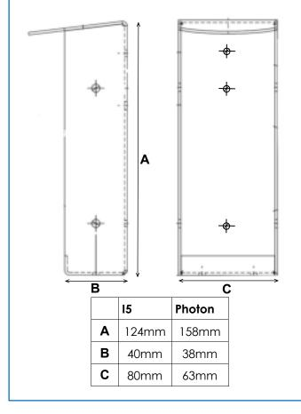
This black powder coated stainless steel cover will also extend the life of the PE beam by offering some protection from the both the weather and vandals.
