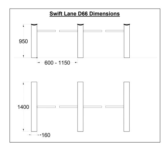
**NOTE:** The concrete pad should be 20Mpa (min) 150 mm thick, cured for 7 days on a suitably compacted foundation. Hold down anchors (4) to be 12mm dia x 100mm into the concrete. Control panel in Entry Leg of Turnstile.
