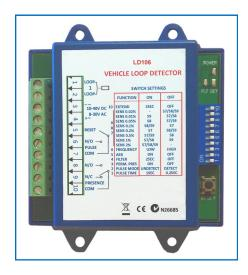
The LD106 can be configured for low power operation making it suitable for use with a solar panel. The detector consumes less than 2mA of supply current when there is no vehicle on the loop.
